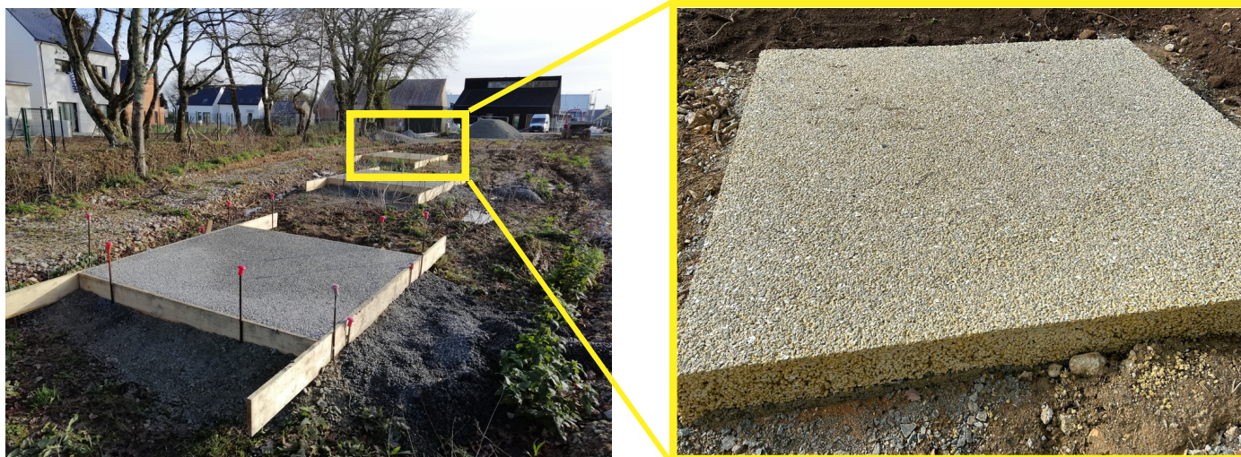
Photograph of the three test boards with zoom (right) of the ochre board chosen for the rest of the work. Picture credit: Golfe du Morbihan Vannes Agglomération (GMVA)
